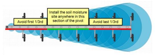
On a 400m pivot the last tower travels approximately seven times faster than the first tower. To ensure the application depth is the same across the length of the pivot, the application rate (mm/hr, or how fast water arrives at the soil surface) increases with the length of the pivot. The inner spans have a low application rate and should be avoided as a soil moisture monitoring site.
