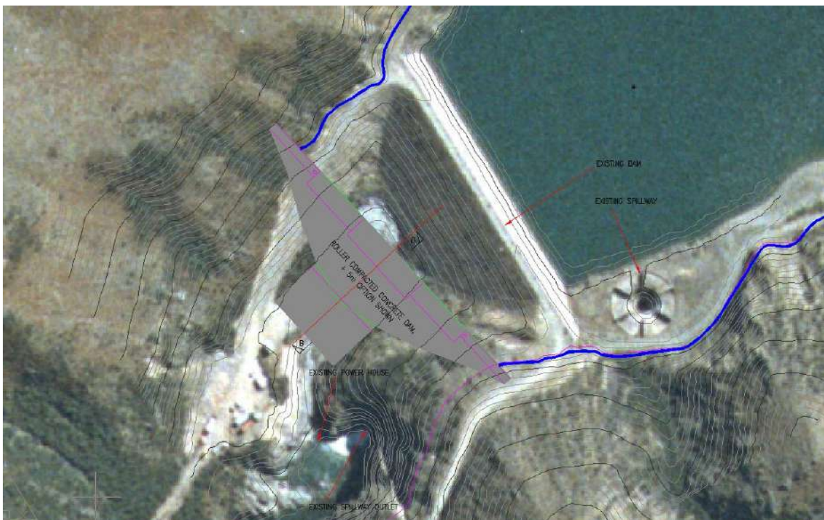
Figure 2 Previous (+5m) RCC Replacement Dam Layout Concept
