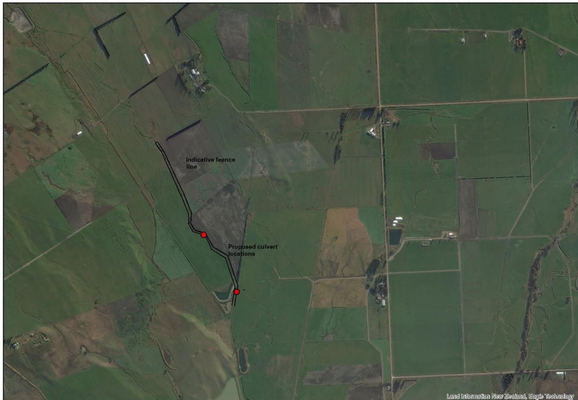
Figure 5 Proposed fence line boundaries and culvert locations
